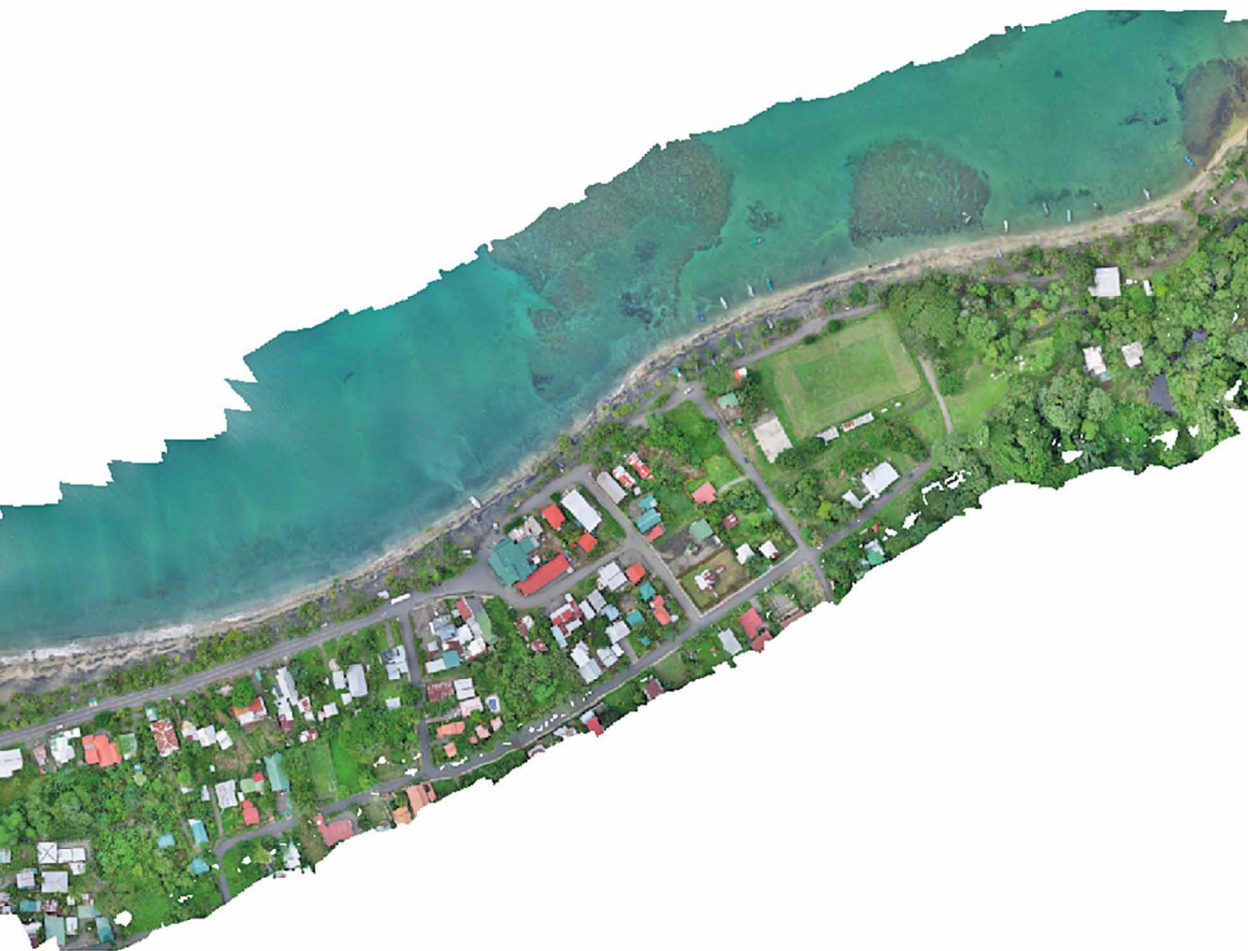
Figure 8.4. Photomosaic constructed from photogrammetric flight at Gando-ca beach. This sector shows intense erosion; note the proximity of infrastructure such as urban facilities, including tourist establishments (such as hotels and restaurants), as a result of the receding coastline.
